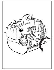
CAUTION! Contact your servicing dealer, if the idle speed setting cannot be adjusted so that the cutting attachment stops. Do not use the machine until it has been properly adjusted or repaired.
